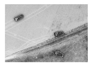
Sherman-DD tanks moving south from Asnelles, behind JUNO beach, on D-Day. Each tank has an enclosing 'skirt', now lowered, which enabled it to swim ashore from a landing ship.
